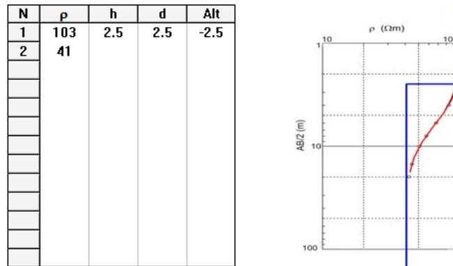
Fig. 5. Diagram of probe S-3 on profile 1
