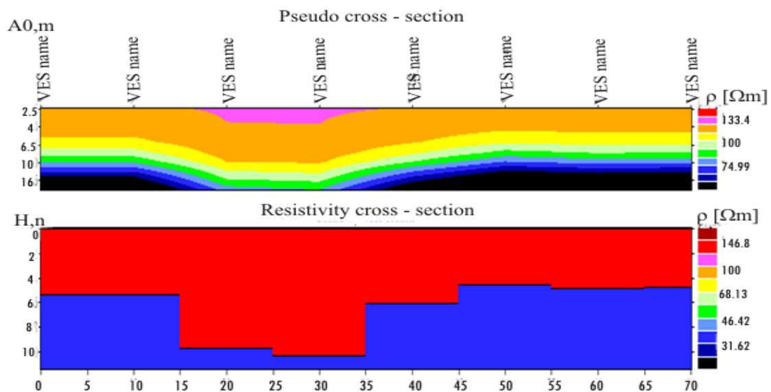
Fig. 6. Geoelectrical model of profile 1
