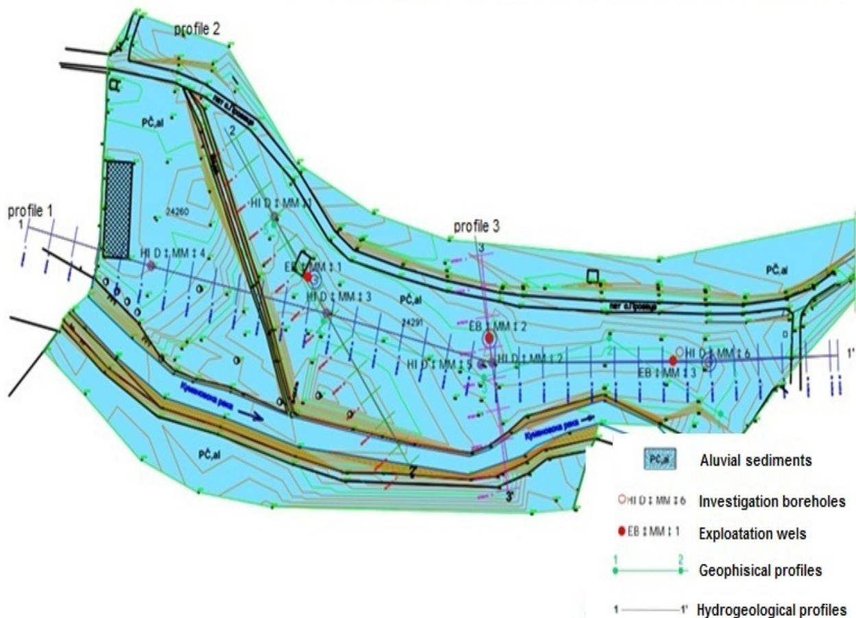
Fig. 3. Hydrogeological map with presented boreholes and wells at a locality "Mitev Most"
