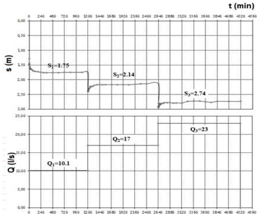
Fig. 6. Dependence of lowering and yielding from time S, Q = f(t)
