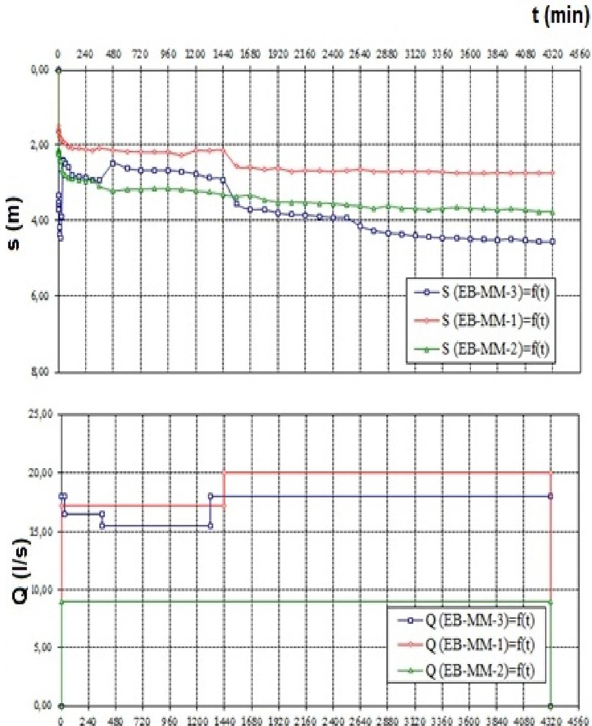
Fig. 7. Dependence of lowering and yielding from time  $S, Q = f(t)$  from group pumping
