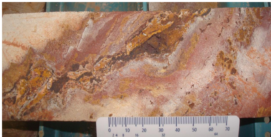
Fig. 3. Intensely altered volcanic rock transformed into quartz-alunite-kaolinite aggregates cross-cut and impregnated by Fe-hydroxides. Illustration of cut drill core from drill hole within the Plavica ore deposit
