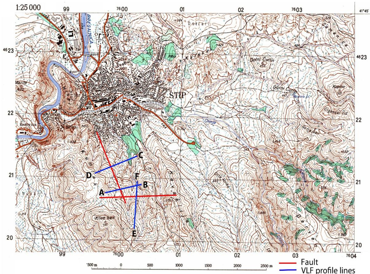
Fig. 2. Topographic map 1:25 000 for the locality "Mazgi", Štip, with field position of prospective VLF electromagnetic investigations
