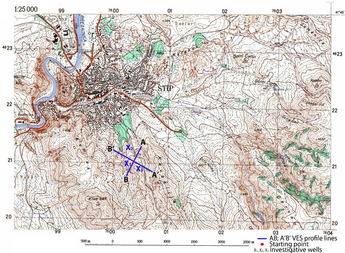
Fig. 6. Topographic map 1:25 000 for the locality "Mazgi", Štip, with field positions of geoelectrical investigations (vertical electrical sounding method)
