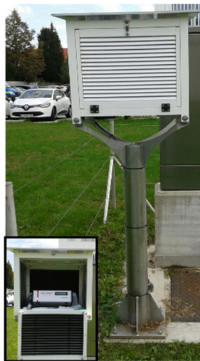
Fig. 1. The weather instrument shelter with the AlphaGuard monitor inside at the meteorological station Ljubljana Bežigrad located at the Environmental Agency of the Republic of Slovenia
