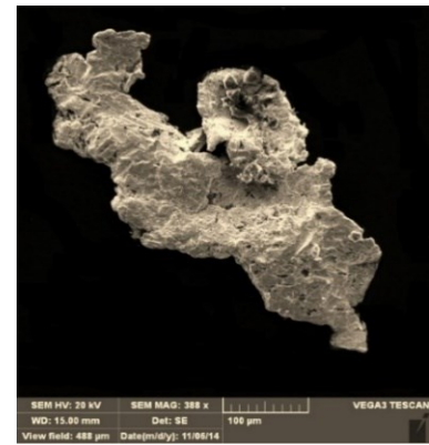
3. Porous partially rounded gold grain
