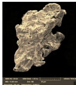
K2.9: Gold grain showing complex partially rounded surface morphology
