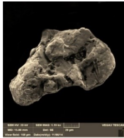
K1.1: Gold grain showing complex partially rounded surface morphology
