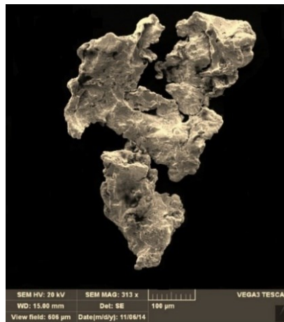
F5. Irregular porous partially rounded gold grain
