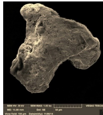
J1.8: Gold grain with well rounded corners and edges
