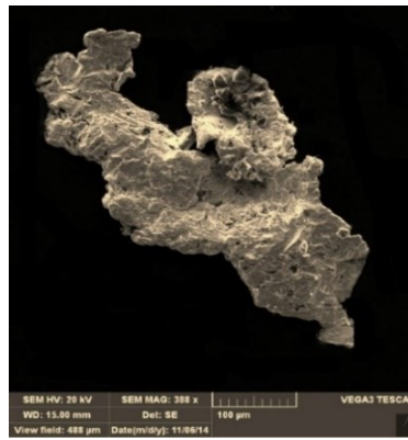
2. Porous, flattened, partially rounded gold grain
