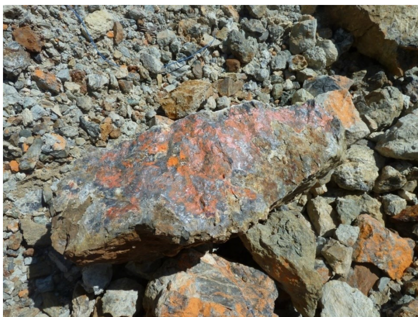
Fig. 2. Large realgar-stibnite ore boulder on the largest dump. Photo T. Đ. in April 2018
