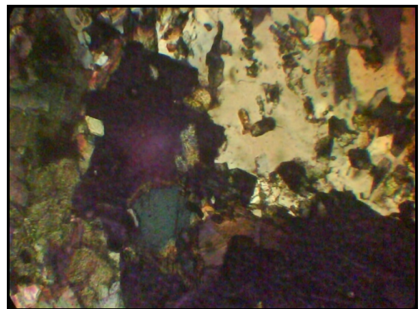
Fig. 5. Microphotography of the amphibolic quartzdiorite of the Kosovska river locality. Crosswise nicols, magnified 10×.
