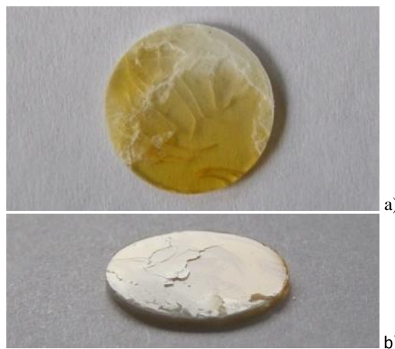
Fig. 1. Pellet made from polycrystalline sample of RbFeSD. All pellets were transparent (a) with glossy and reflective surface (b).
