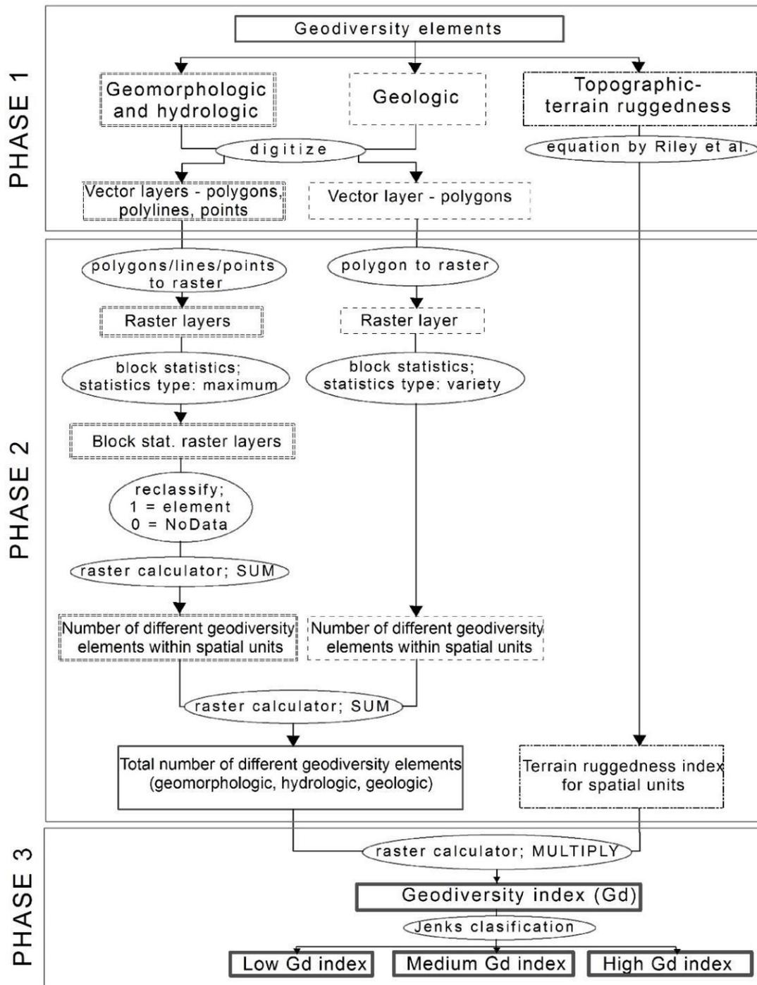
Fig. 2. Detailed scheme of geomatics – GIS based system for inventory and evaluation of geodiversity
