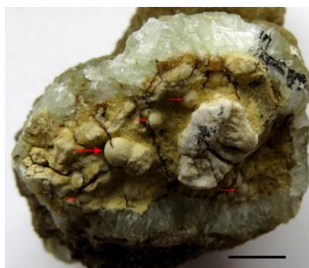
Fig. 8. Magnesite (±silica) globules on a surface of magnesite nodule with dolomite encrustation. The largest arrow pointing the one 2.35 mm in diameter. Size bar 5 mm.
