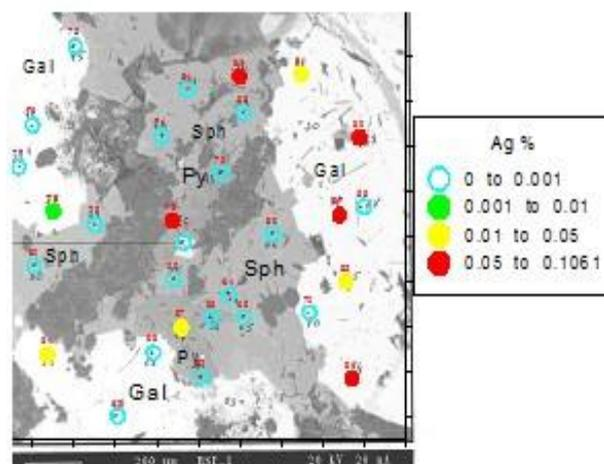
Fig. 8. Contents of Ag, H5-polished section [5].
