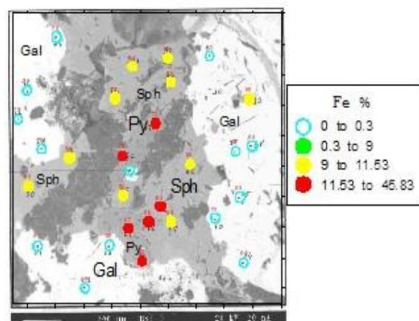
Fig. 9. Contents of Fe, H5-polished section [5].
