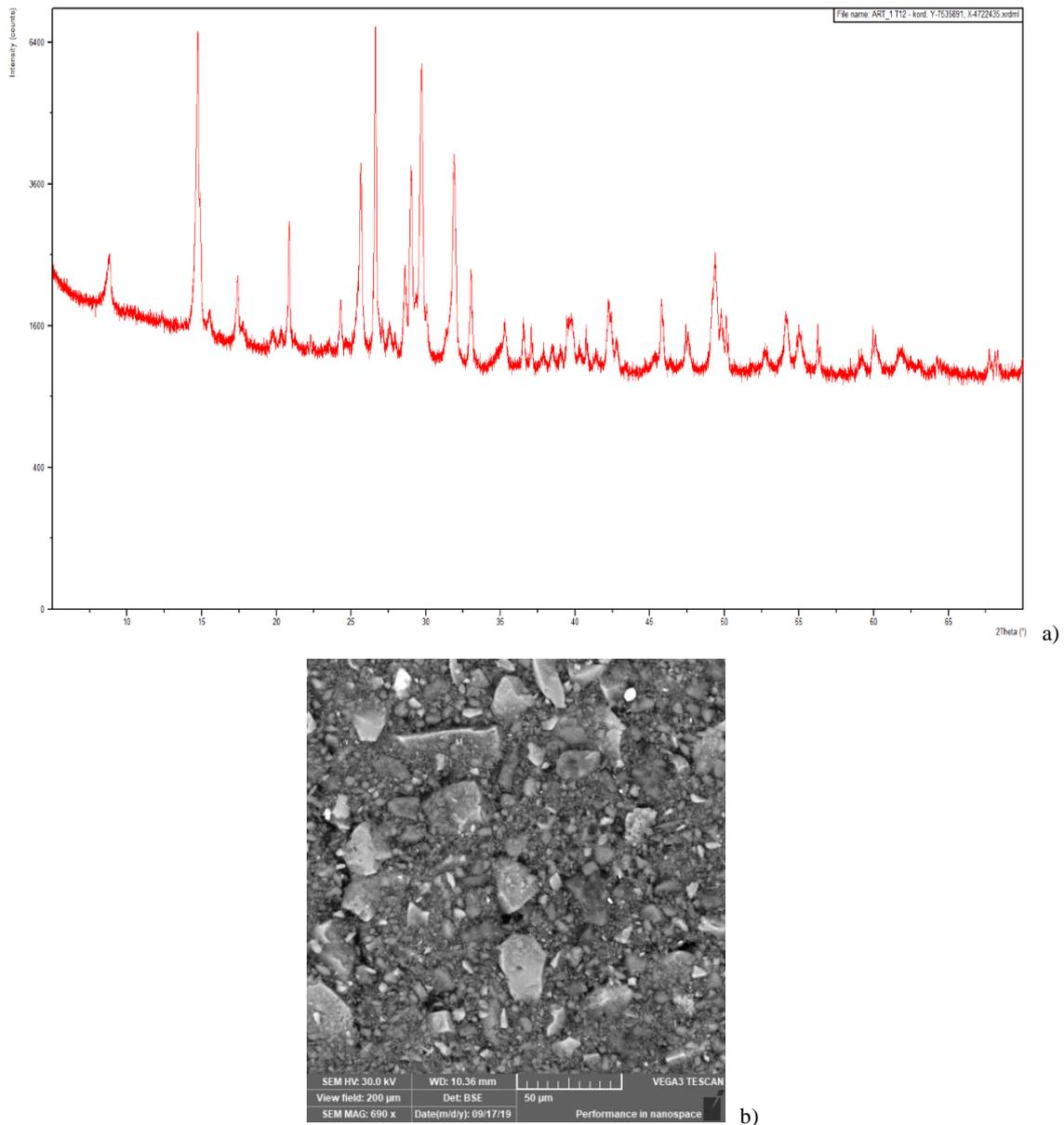
**Fig. 5.** XRPD spectrum (a) and SEM-BSE photomicrographs (b) of the tailing sample T12
