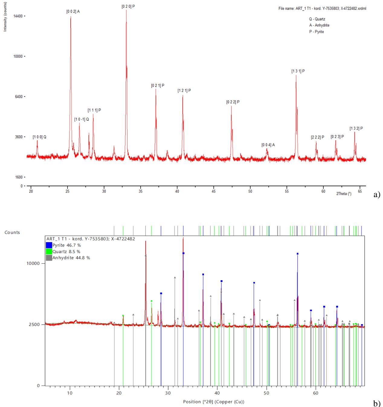
**Fig. 4.** XRPD spectrum of tailing sample T1 characterized by: a) Miller indices, b) percentage composition
