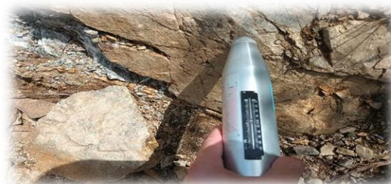
Fig. 2. Sclerometer test point in leucocratic granite
