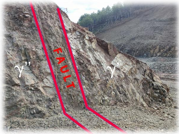
Fig. 8. Tectonic border between \gamma'' highly fissured and \gamma' medium fissured gray granites
