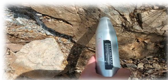
Fig. 2. Sclerometer test point in leucocratic granite
