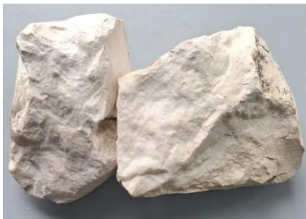
Fig. 6. Macroscopic features on magnesite from the Pčinja river area
