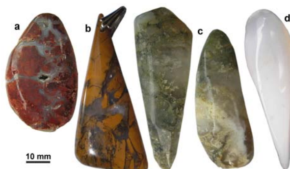
Fig. 9. Baroque gems obtained by the experimental processing of various gemstone types from Gaj-Lazine deposit:
