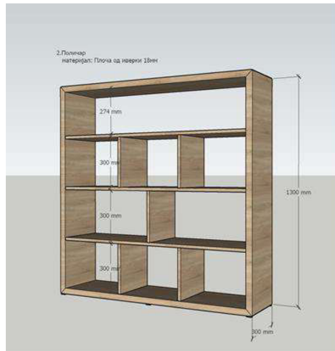
Figure 2. 3D model of a free-standing shelves rack, prepared in SketchUp, 3D interior design software, through the classic way of production preparation
