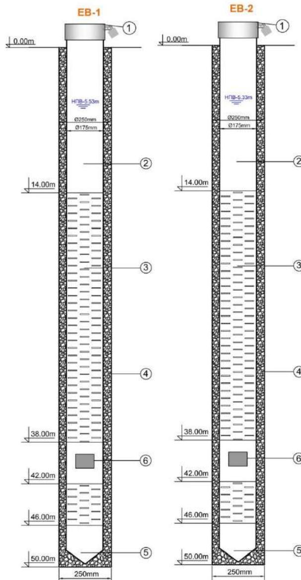
Figure 3. Schematic construction of exploitation wells EB-1 and EB-2
