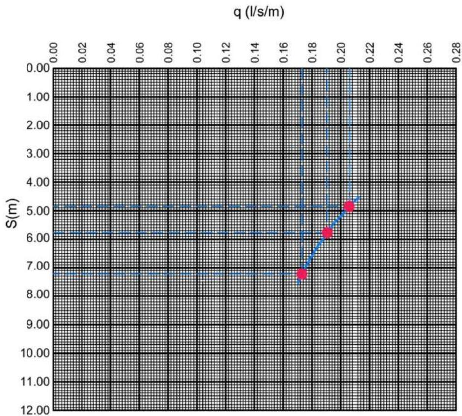
Figure 5. Diagram of specific yield  $q = f(S)$  for exploitation well EB-1
