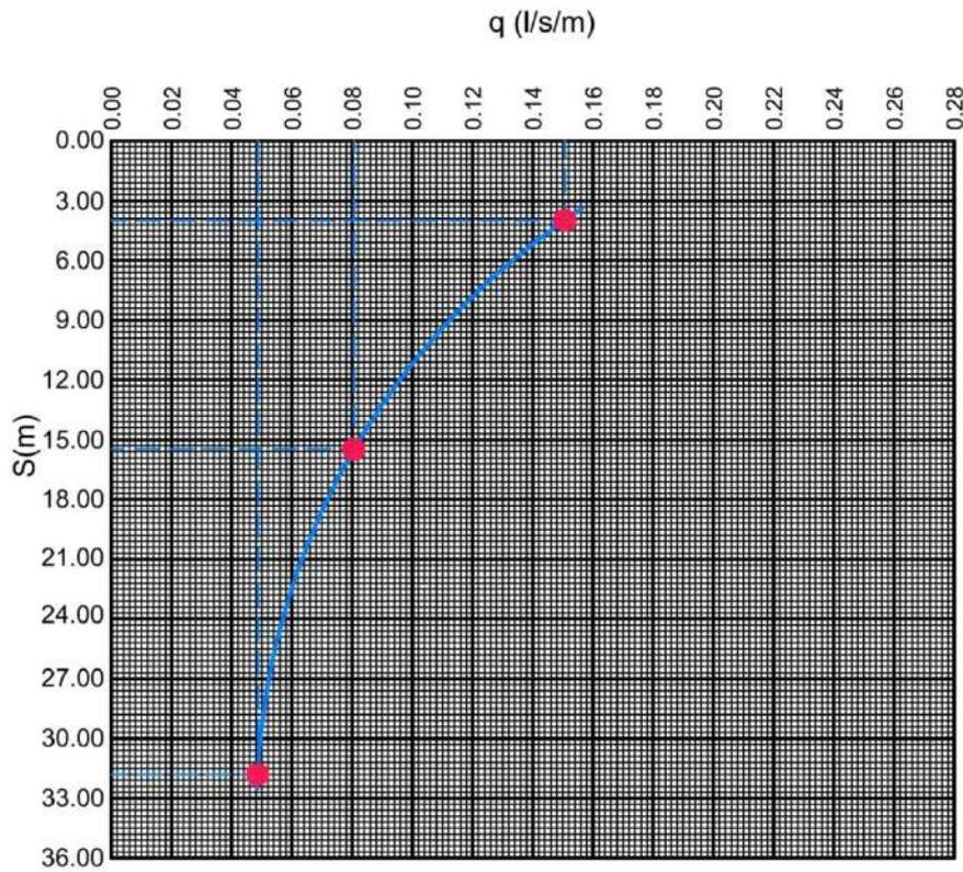
Figure 7. Diagram of specific yield  $q = f(S)$  for exploitation well EB-2
