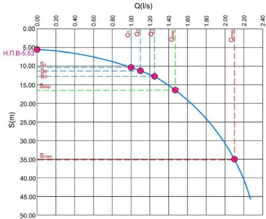
Figure 4. Diagram of dependence of yield depending on  $Qf(s)$  lowering for exploitation well EB-1
