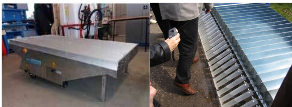
Figure 5. A measuring device for horizontal liquid distribution – spray scanner
