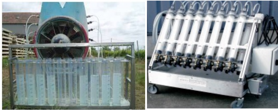
Figure 3. A measuring device for mist blower nozzle flow
