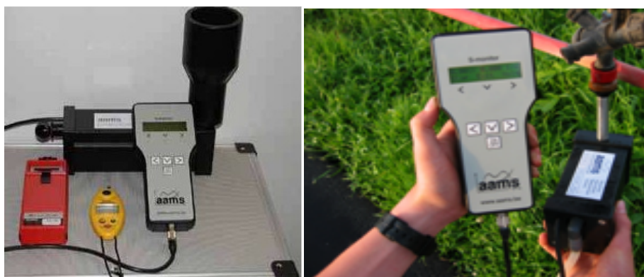
Figure 4. A measuring device for sprayer nozzle flow
