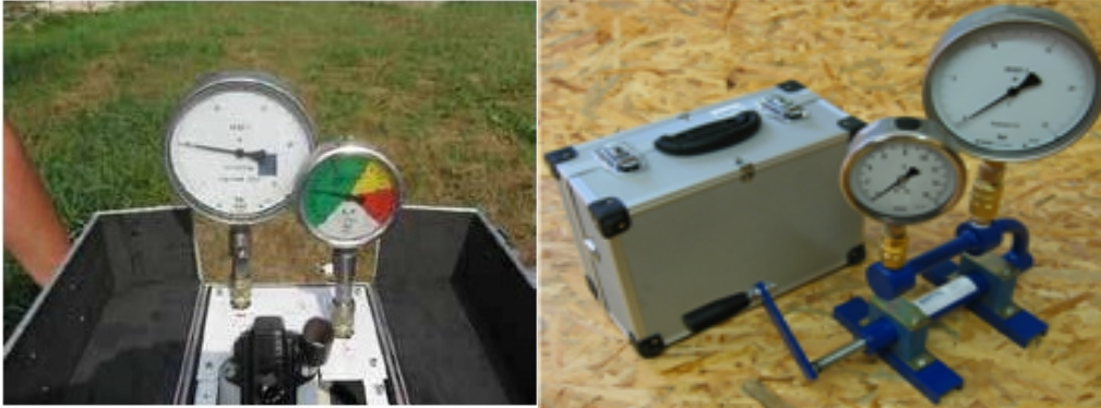
Figure 1. A measuring device for pressure gauge correctness
