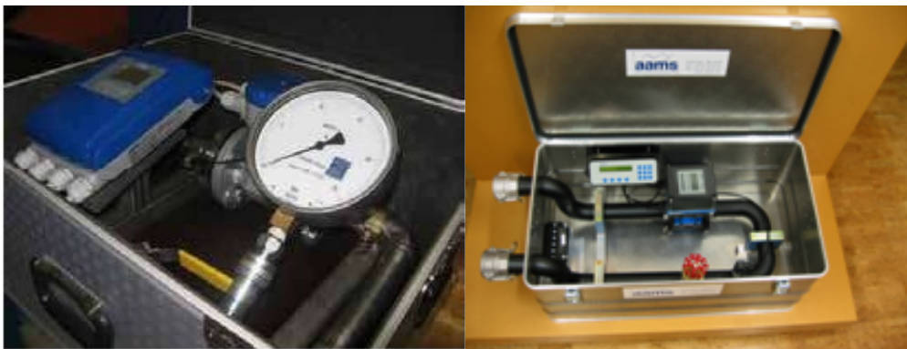
Figure 2. Electromagnetic device for pump flow measuring
