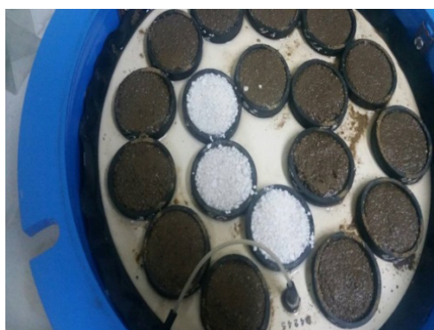
Figure 2. Preparing soil/substrate and placing samples on Bar extractor and Porous plate extractor
