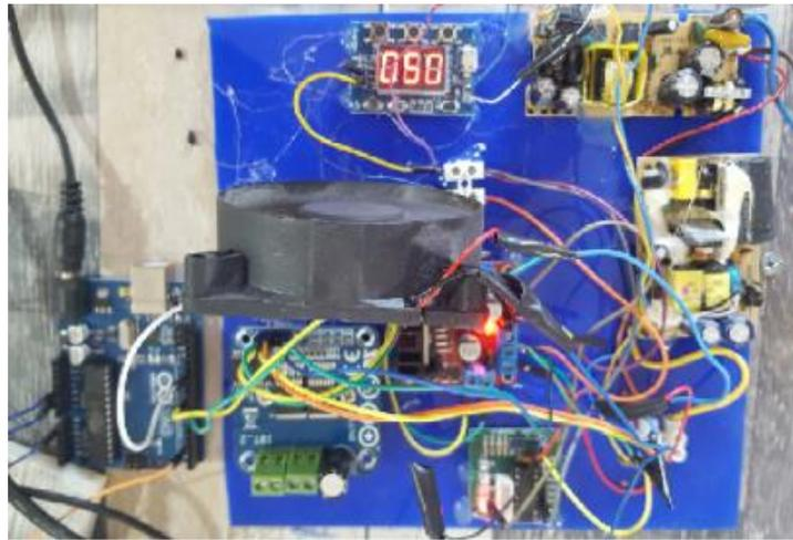
Figure 6. *Amega 328P microcontroller based circuit prototype and BST7960 bridge converter implemented for generating square voltage*
