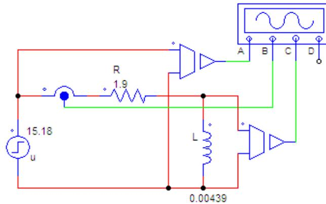
Figure 2. Circuit for simulations in the PowerSim program on RL-circuit supplied by step voltage, turned on at  $t = 0$  s with conditions  $i(0^-) = i(0^+) = 0$  A.
