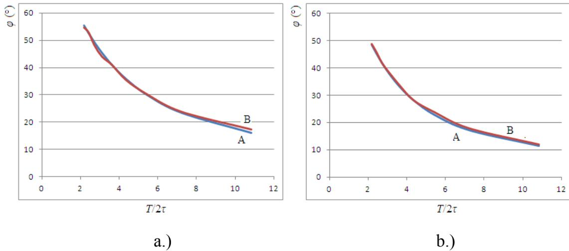
Figure 9. Graph of the phase angle: a.) the sinus supply obtained with the calculation (curve A) by (2) and simulations (curve B) in the PowerSim program and b.) the square supply obtained with the calculation (curve A) by (12) and simulations (curve B) in the PowerSim program
