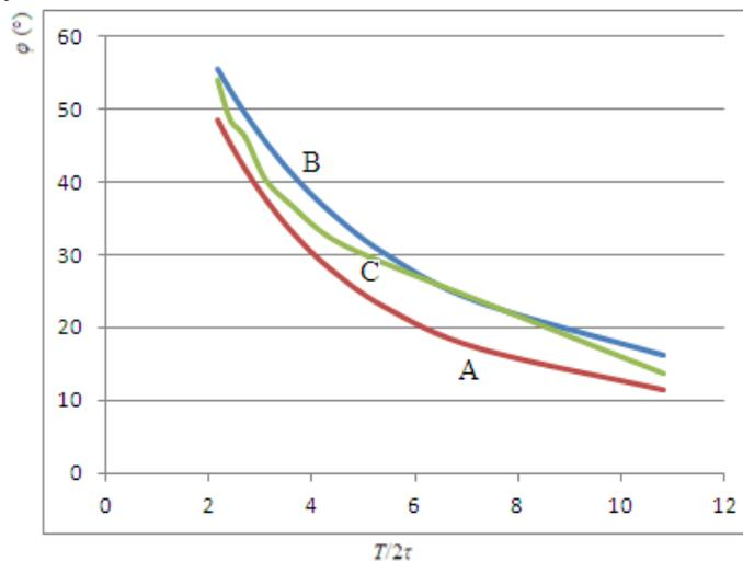
Figure 10. The graphs on the phase angle in RL-circuit for the square supply obtained with the calculation (curve A) by (12), for the sinus supply obtained with the calculation (curve B) by (2) and the experimentally obtained graph (curve C) for the square supply
