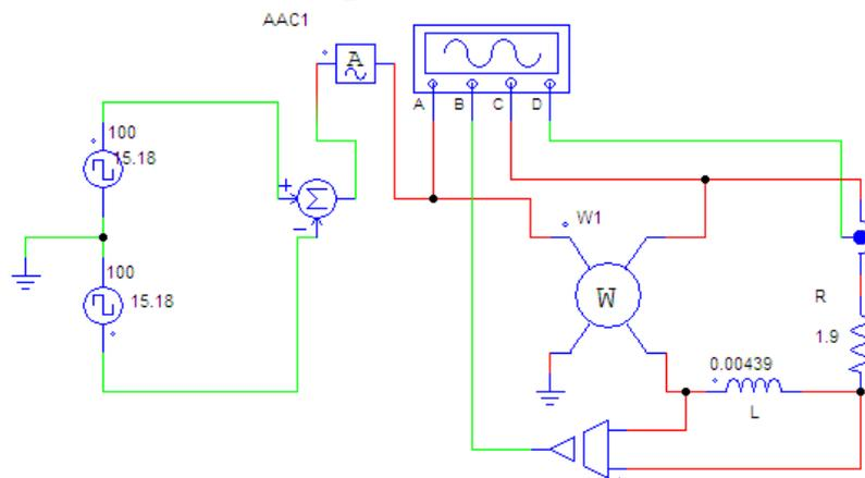
Figure 4.  $RL$ -circuit in the PowerSim program used for determining the phase angle between the voltage and the current, in case of voltage supply with square waveform
