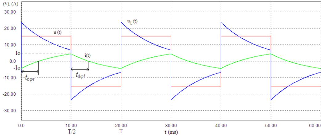
Figure 5. Waveform of the supplying voltage  $u(t)$ , the inductor voltage  $u_L(t)$  and current  $i(t)$  in the circuit from Figure 4, in steady state for the square voltage pulse with switching frequency  $f_s = 50$  Hz, amplitude  $V = 15.18$  V and duty cycle  $D = 0.5$
