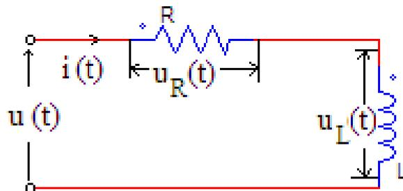
Figure 1. Serial  $RL$ -circuit
