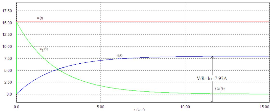
Figure 3. Waveform of the input step voltage  $u$ , the inductor voltage  $u_L$  and the current  $i$  of the circuit from Figure 2 turned at  $t = 0$  s with conditions  $i(0^-) = i(0^+) = 0$  A.
