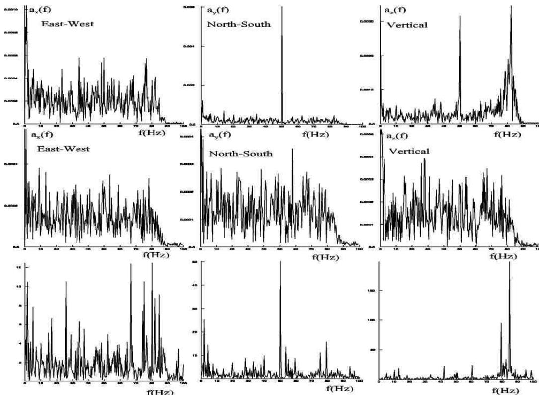
Figure 2. FFT of acceleration  $a(t)$  in three orthogonal directions obtained from the ambient vibration test with two accelerometers EQR 120 at Berovo lake weekend house.
