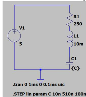
Figure 2. Serial RLC circuit in LTSpice
