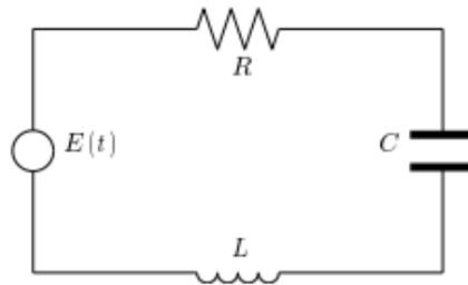
Figure 1. Serial RLC circuit
