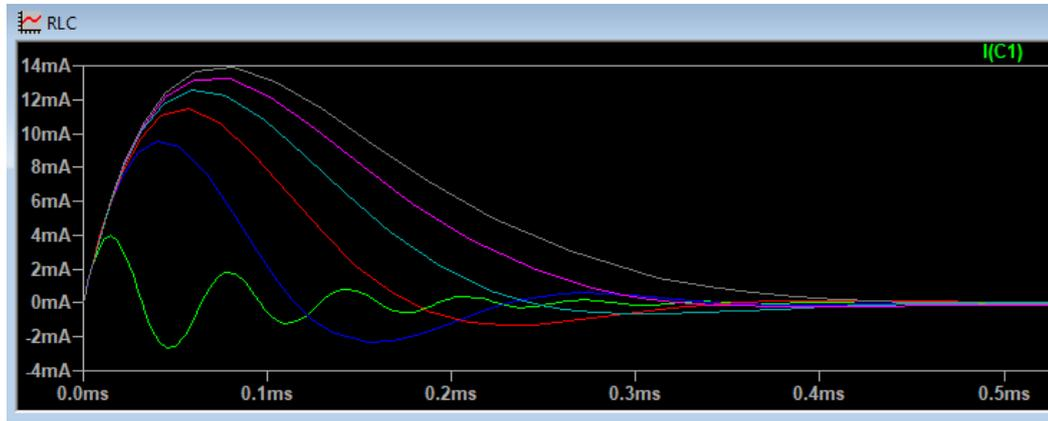
Figure 3.  $R=250\Omega$ ,  $E=5\text{ V}$ ,  $L=10\text{ mH}$ ,  $C$  variable from  $10\text{ nF}$  to  $510\text{ nF}$
