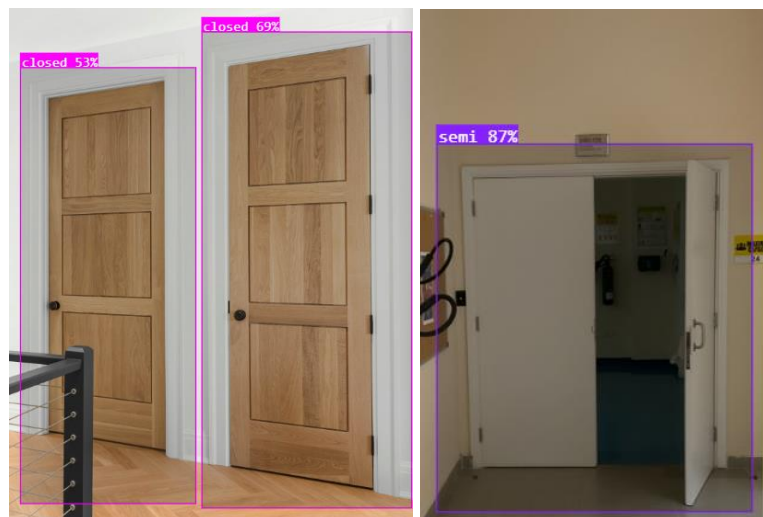
Figure 5. Real-time detection of doors in a sample image.
