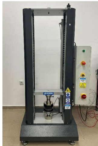
Figure 2. Universal testing machine used for compression testing
