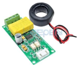
Figure 6. The board of PZEM-004T power meter
