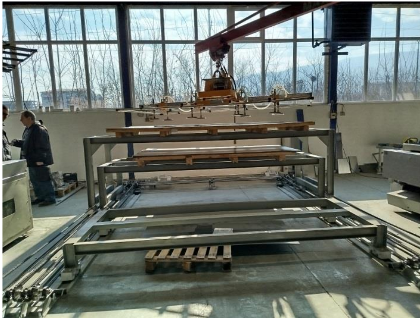
Figure 8. Transversal unit with vacuum handling system.
