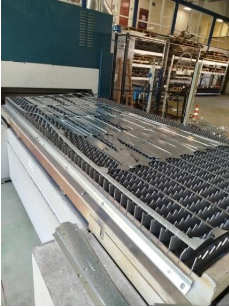
Figure 9. Laser cutting machine and processed sheet metal.
