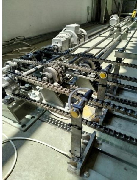
Figure 10. Mechanical transmission system with motor and chain drive.
