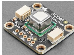
Figure 6. The electronic board on SDC40 CO2 sensor
