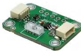
Figure 7. The electronic board on the VEML7700 light sensor
