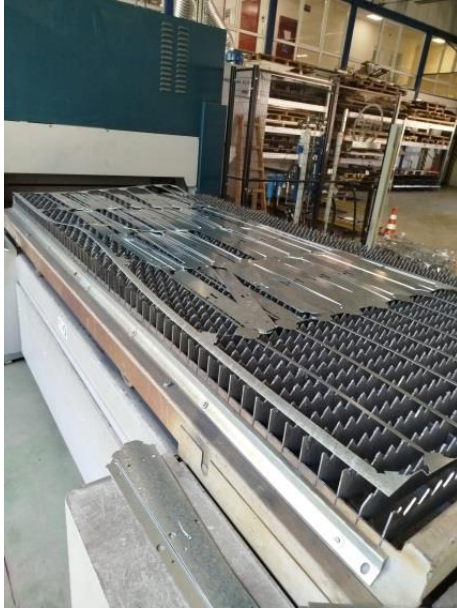
Figure 9. Laser cutting machine and processed sheet metal.
