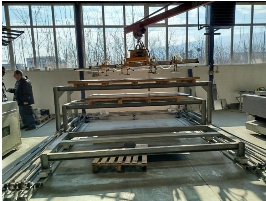
Figure 8. Transversal unit with vacuum handling system.
